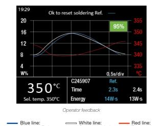
The Soldering Assistant is the solution to optimize repetitive soldering processes, improving your soldering production line with greater quality and control.
