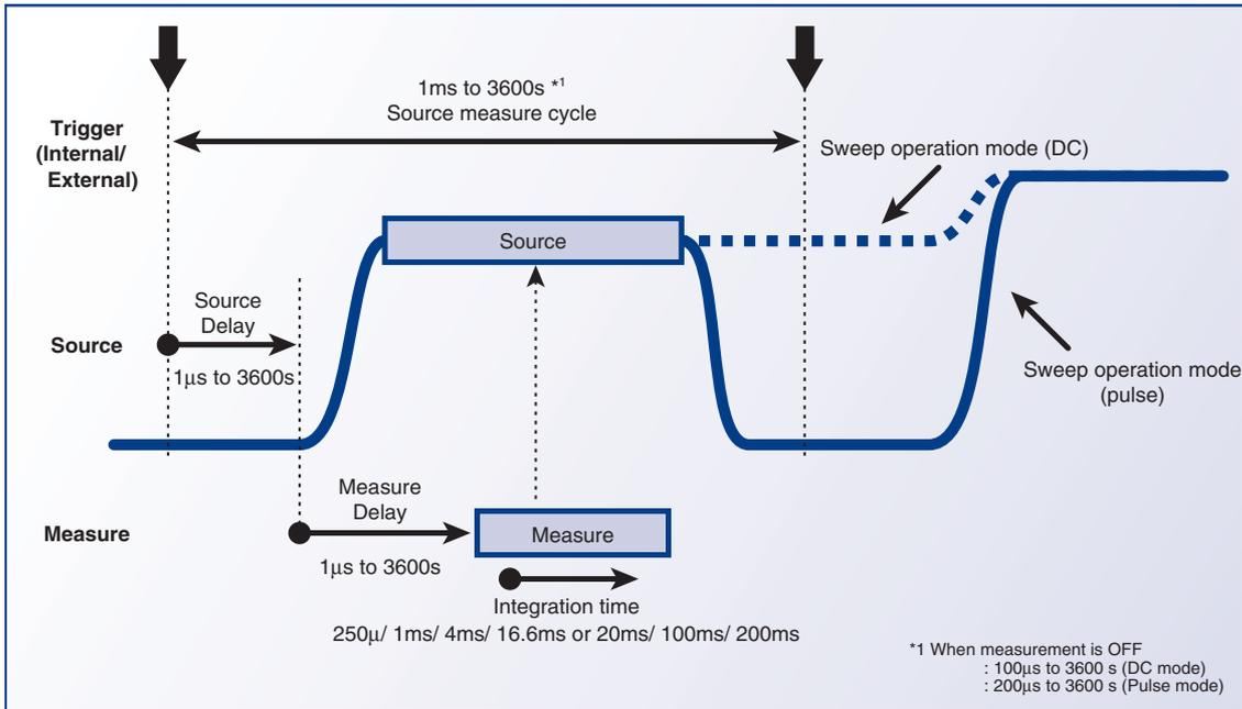
Difference Measurement Using the Sweep Operation
