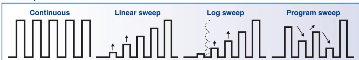
Generation and Measurement Timing (Source Measure Cycle)
